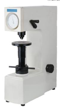
iRock-430H Rockwell hardness tester is a popular-used hardness testing instrument to measure the hardness of the metal materials. No need power supply, the speed of the test force loading is regulated by the buffer and the test force is regulated by the load-change hand wheel. It has easy operation and stable performance, therefore it is widely used.
